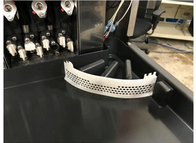
*The following illustrates the steps necessary to install a drain strainer to Lancer Cold Carbonated Ice Cooled Drop-In Dispensers, in order to reduce the chance of clogging the drain.*
