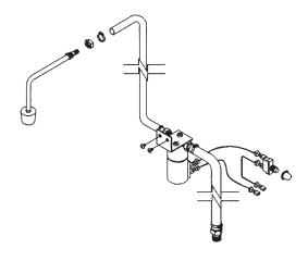
Water Spigot for Ambient Temperature Water Kit PN 82-3801 for 2200
