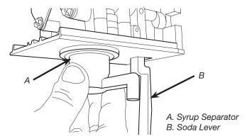
Using a Lancer ratio cup, activate the valve and capture a sample. Verify that the syrup level is even with the water level. Use a screwdriver to adjust if needed.
