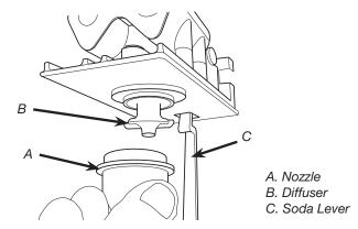
3. Remove the diffuser by pulling down.
