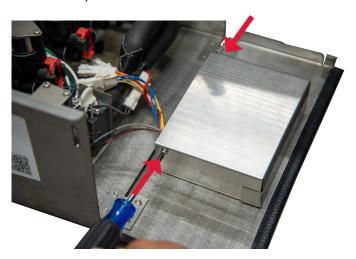
11. Close and secure door ensuring wires are clear of pinch points.
