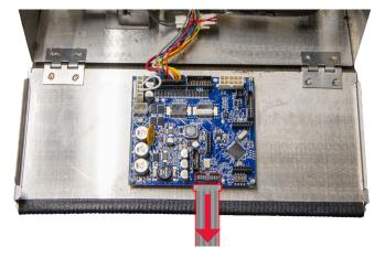
2. Detach PCB from standoffs by pushing in standoff barb to release board.
