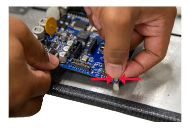
3. Remove all four standoffs from door by pushing in standoff barbs to release.
