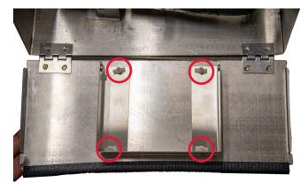
6. Press standoff barbs into PCB holes until secure.
