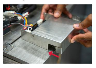
10. Using the two (2) provided Phillips screws (04-1749/01) secure enclosure cover to base.
