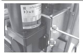
10. Slide the Motor and Mounting Plate Assembly off the Auger Shaft.
