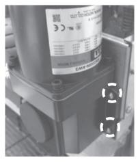
14. Screw new capacitor into Control Box and connect new Harness to Capacitor, PCB, and Motor.
