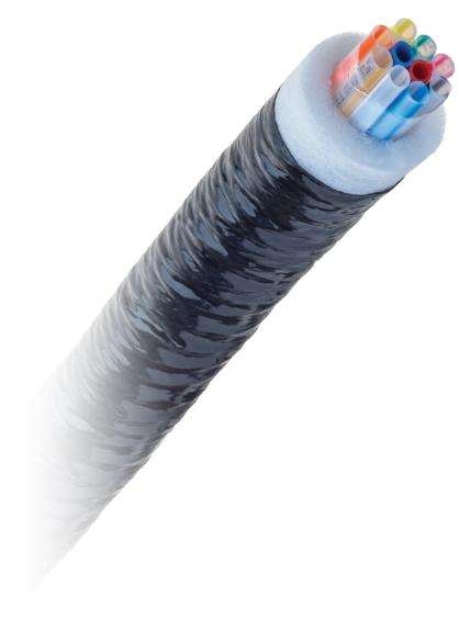
**kōld Seal** non-cabled and cabled insulated bundles are comprised of flushable **kōld Seal** tubes. Each tube is color-coded and individually numbered, and strategically placed around red/blue-colored coolant tubes to provide optimum cooling and flavor protection.
