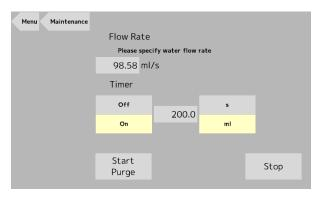
Using the keypad, enter a specific volume to be dispensed based on the size of the graduated cylinder being used to calibrate the plain water module.
