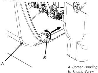
7. While holding the plastic screen housing, tilt the housing forward until the housing disengages from the unit.
