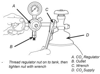
2. Connect a 3/8" nut, stem and seal to CO<sub>2</sub> regulator outlet.
