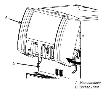
2. Rotate the merchandiser, away from the unit, from the bottom then lift the merchandiser straight up to detach from the top of the ice bin and remove from the unit.
