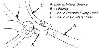
10. Route appropriate tubing from the remote pump deck outlet to the carbonated water inlet at unit.
