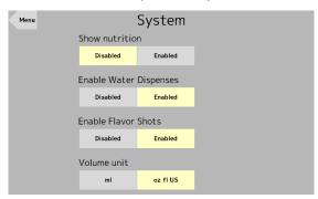
Press the Enabled button, below the "Enable Water Dispenses" heading, to have the ability to pour plain/ carbonated water from the main screen.
