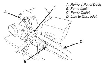
Install a shut-off valve in the water line feeding the remote pump deck as well as the water line feeding the plain water inlet. 12. Route appropriate tubing from the syrup pump location to the syrup inlets and connect tubing to all syrup inlets.
