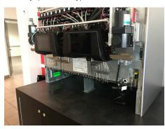
Install the new extended splash plate (51-7039), included with kit, to the front of the unit.
