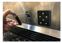
Disconnect the ADA Panel harness and remove from the unit. Repeat Steps 1 - 4 for second ADA panel.
