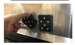
Carefully pull ADA panel and electric wire harness from the unit's splash plate, until the harness connector is visible.
