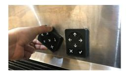
Carefully pull ADA panel and electric wire harness from the unit's splash plate, until the harness connector is visible.
