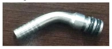
The old stainless steel tube fitting has "machined-in" barbs with rounded/flat edges. The outer diameter of these fittings can range from 0.273 inches to 0.283 inches.
