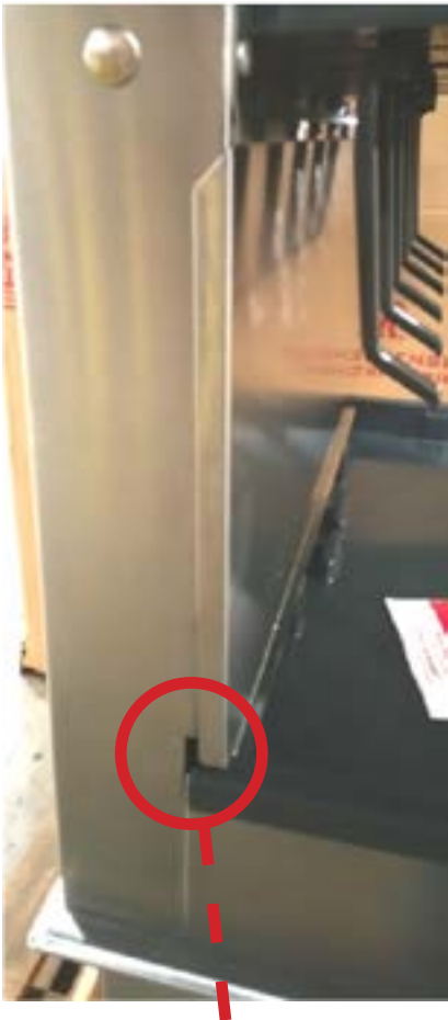
Small gap caused by mis-aligned drain tube
