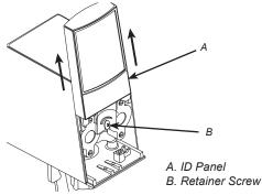
If attached to unit, disconnect valve wire harness, close the valve stems on the backblock, and lift the retainer clip to remove valve from unit.
