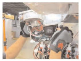
3. Cut the existing power cord and remove from unit.
