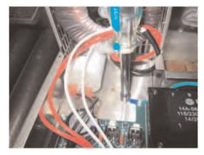
9. Insert bushing with cord into the power supply.
