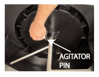
Remove the agitator pin clip and pin.
