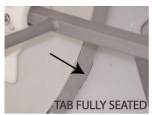
Ensure the tab at the bottom of the shield aligns with the slot at the bottom of the ice shroud. Ensure the tab fully seats.
