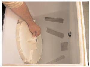
Install the pellet dispensing wheel. Ensure pin holes are aligned.
