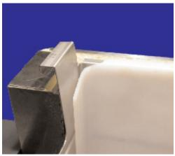
Slide the shield into the ice shroud ensuring the shield is captured between the ice shroud and the ice bin at the top left and right corners. Above is a detailed view.
