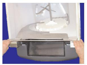
Install the shield. Hold the shield so that the hooks are facing the front of the machine.
