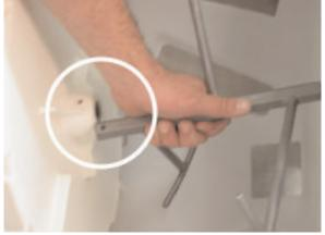
Install the pellet agitator assembly: insert the end of the agitator into the bearing on the back wall. Push agitator towards rear to allow clearance between the agitator and wheel hub. Align agitator pin hole with wheel pin hole. Fit agitator to the wheel hub.
