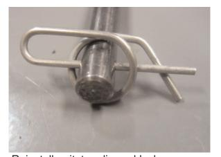
Reinstall agitator clip and lock.
