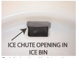
Push the ice shroud back towards rear wall so that the ice chute clears the top wall of the ice bin. Push the ice shroud into the ice bin. Ensure the ice chute fits into the ice chute opening in the ice bin.
