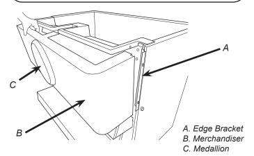
16. Using the four (4) bracket screws provided, install the merchandiser to the unit.
