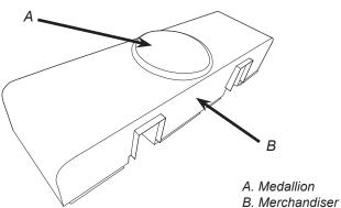
14. Using the two (2) medallion screws provided, install the medallion to the front of the merchandiser by screwing in the screws to the back of the merchandiser.
