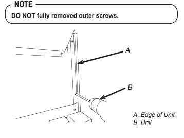
10. Slide the two (2) brackets provided over the outer screws loosened on the previous step. Make sure to install the appropriate bracket to each side of the unit.
