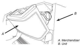
5. Unplug the low ice indicator cable inside the merchandiser on the left side of the unit, before removing the merchandiser.
