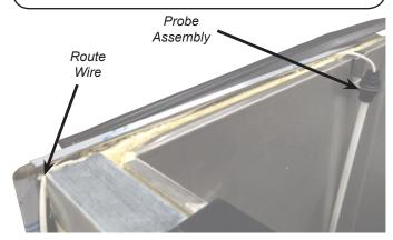
8. Install edge guard to the edge of the sheet metal where the probe assembly wire first becomes exposed at the front of the unit. This will prevent the sheet metal from pinching or cutting the wire.
