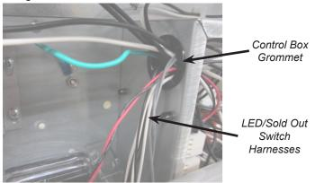
9. Plug the grey sold out switch harness and the red and black LED harness into the control box in the connections shown on the wiring diagram.
