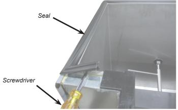
3. Continue prying up seal all the way around to the back of the unit.
