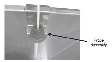
6. Using the knife or box cutter, score and remove the foam along the edge of the ice bin.
