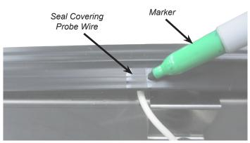
11. Lift the seal and score the bottom portion of the seal between the markings created in the previous step.
