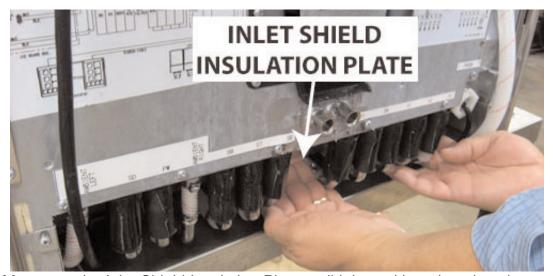
Manuever the Inlet Shield Insulation Plate until it is positioned against the angled surface of the inlet shield. Ensure the Inlet Shield Insulation Plate is positioned in between the brackets.
