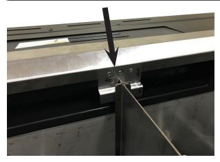
4. Install any necessary Vertical Filler Plates to either side of Adapter Base.
