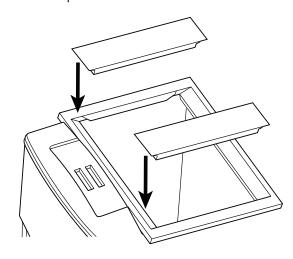
Install any necessary Horizontal Filler Plates to top of Vertical Filler Plates in order to fit the unique connection between the icemaker and the dispenser.
