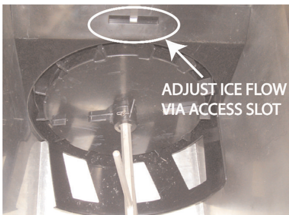
13. If at a later date you need to re-adjust the ice flow, you can do so via the access slot in the top of the wheel shroud. You do not need to disassemble the wheel assembly.
