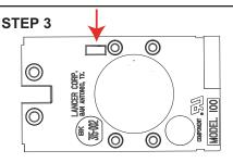
For new bottom plates, use a screwdriver to rupture the rectangular hole on right side of bottom plate. Smooth edges. Skip to step 5.
