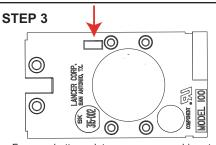
For new bottom plates, use a screwdriver to rupture the rectangular hole on right side of bottom plate. Smooth edges. Skip to step 5.
