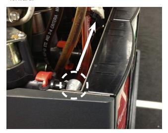
Inspect the larger 25-pin cables connected to the Touch Panel. If unit has a short pigtail with four (4) wires, the Valve Cable Harness does *NOT* need to be replaced.
