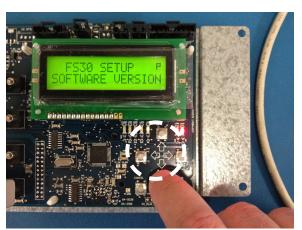
Press the enter key to see the current SW versions for the valve boards. By using the up or down arrow button you can change the valve touch pad number to see which software version it has. Verify all valve boards are current by pressing the up or down to view entire list.
