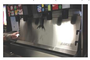
5. Install the Pendants on the Splash Plate by sliding them into the slot, as shown below.
