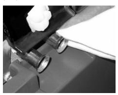
Slightly pinch the new elbow fitting (Lancer PN: 05-3192) to form an oval shape.
