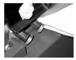
Slightly pinch the new elbow fitting (Lancer PN: 05-3192) to form an oval shape.
