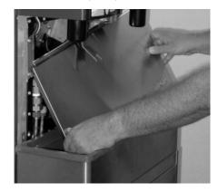
3. Pinch the shorter drain elbow and pull away from the drain spout to remove from unit.
