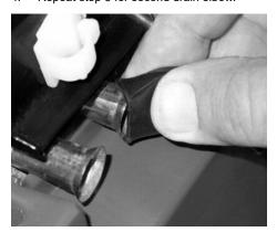
The following illustrates how to replace the existing, shorter drain elbow fittings (Lancer PN: 05-2771) with the new, longer drain elbow fittings (Lancer PN: 05-3192).
