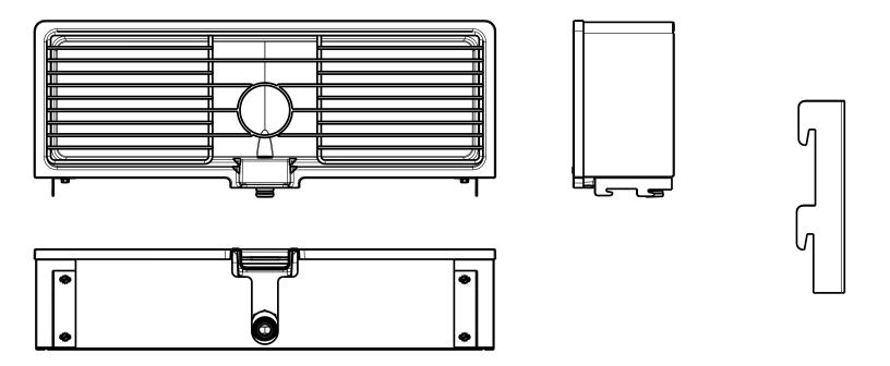
WHEN REPLACING THE LEGACY (PRE-2003) DESIGN HOOKS: REMOVE EXISTING HOOKS FROM DRIP TRAY ASSEMBLY AND REPLACE WITH 30-10644 AND 30-10645 AS SHOWN.
