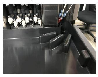
2. Position the drain strainer, with teeth up, around the outer edge of the corner drain as shown below:
