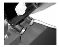
4. Slightly pinch the elbow fitting to form an oval shape.
