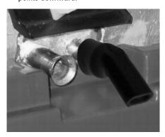
8. Install the second elbow fitting onto the open drain tube.
