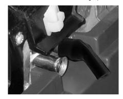
Rotate the elbow fitting so that the exhaust points downward.
