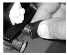
6. Push the elbow fitting back over the drain tube until flare reaches the angle point.
