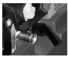
7. Rotate the elbow fitting so that the exhaust points downward.
