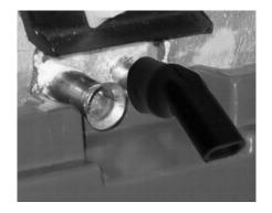
. Install the second elbow fitting onto the open drain tube.
