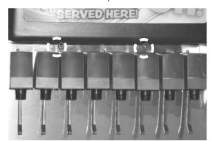
Use a Phillips Screwdriver to remove the Auger Motor Shaft Cover from the Auger Motor gear head.
