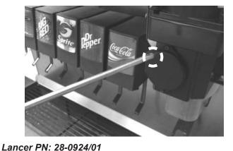
5. Remove the Clip from Auger Motor Shaft.
