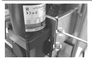
8. Slide the Motor and Mounting Plate Assembly off the Auger Shaft.
