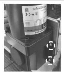
12. Reinstall the Shaft clip and the Shaft cover. If the groove for the clip is not visible, the Shaft can be moved by pushing on the Shaft Clip between the Motor and the Ice Chute.
