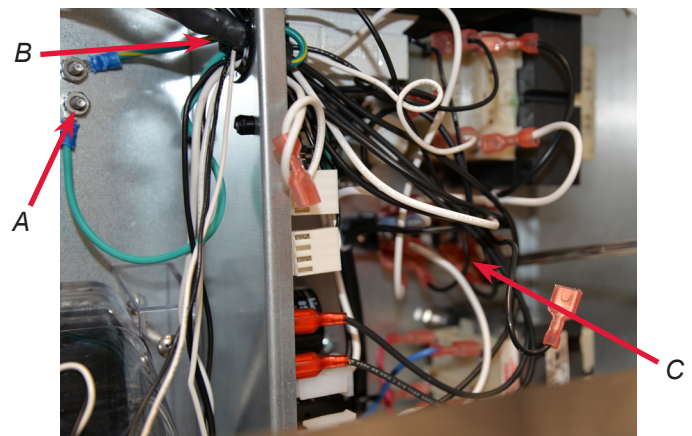
A. Ground Connection B. LED Driver Cables C. Power Strip
