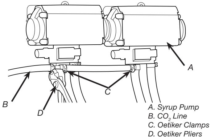
3. Using tubing cutters, cut the CO<sub>2</sub> supply line to the syrup pumps and install tee fitting. Then, route the appropriate tubing from the tee fitting to the syrup pumps and to the unit.
