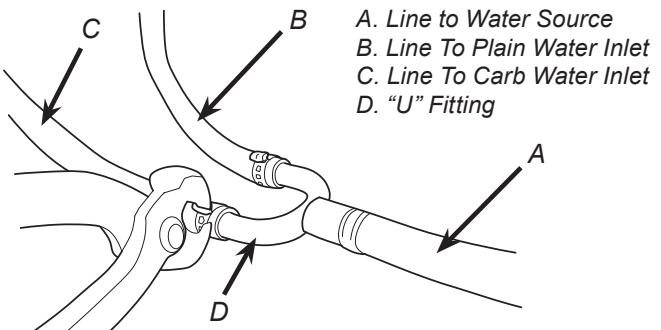
18. Route appropriate tubing from the plain water inlet, located at the front of the unit, to one side of the "U" fitting at water supply and connect tubing to inlet.
