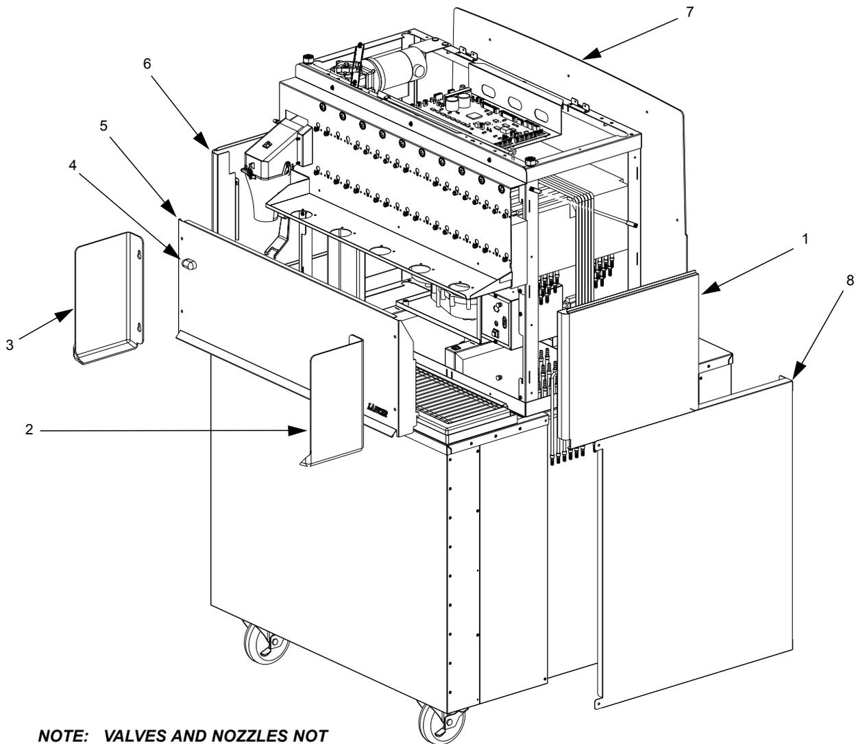
**NOTE: VALVES AND NOZZLES NOT SHOWN FOR CLARITY**
