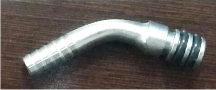
The old stainless steel tube fitting has "machined-in" barbs with rounded/flat edges. The outer diameter of these fittings can range from 0.273 inches to 0.283 inches.
