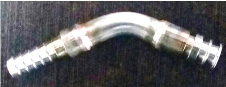
The upgraded fittings are "machine bar stock" with much more aggressive designed barbs to give more clamp ring force application to the red-line tubing of the dispensers.
