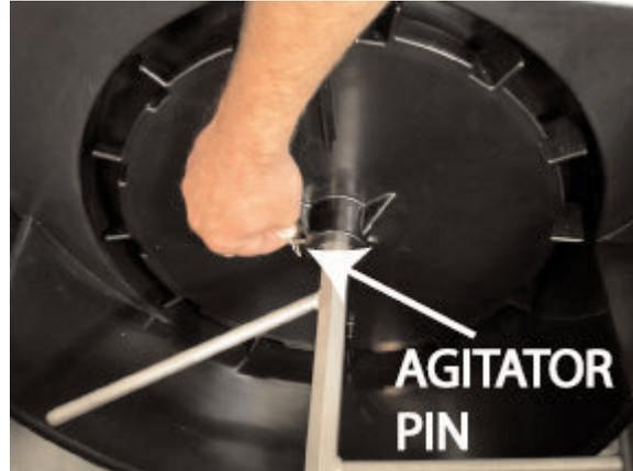
Remove the agitator pin clip and pin.
