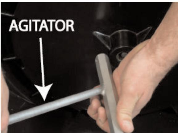
Remove the cube agitator bar. Push the agitator towards the rear of machine to disengage it from the wheel. Pull the agitator to the side to clear the wheel hub.
