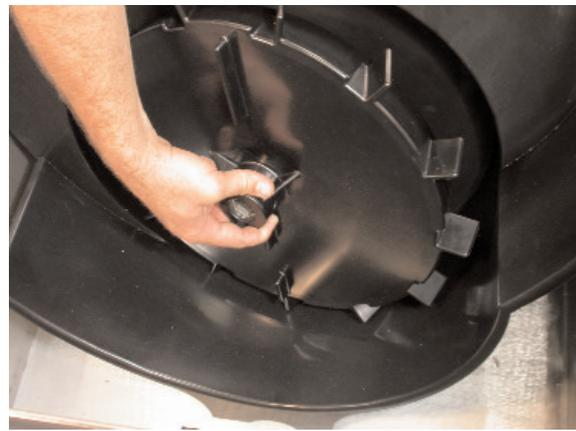
Pull the agitator towards the front of the machine to disengage from the back bearing. Remove the cube dispensing wheel.
