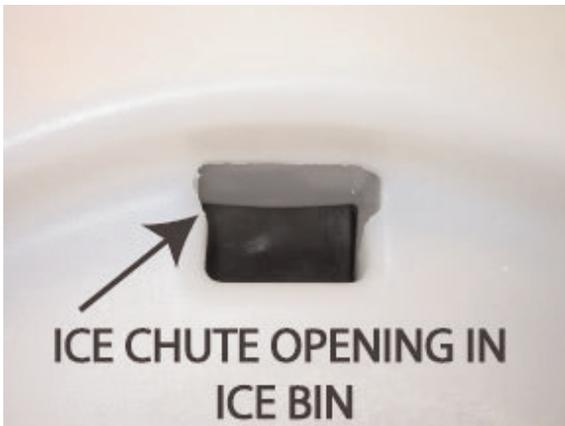
Push the ice shroud back towards rear wall so that the ice chute clears the top wall of the ice bin. Push the ice shroud into the ice bin. Ensure the ice chute fits into the ice chute opening in the ice bin.
