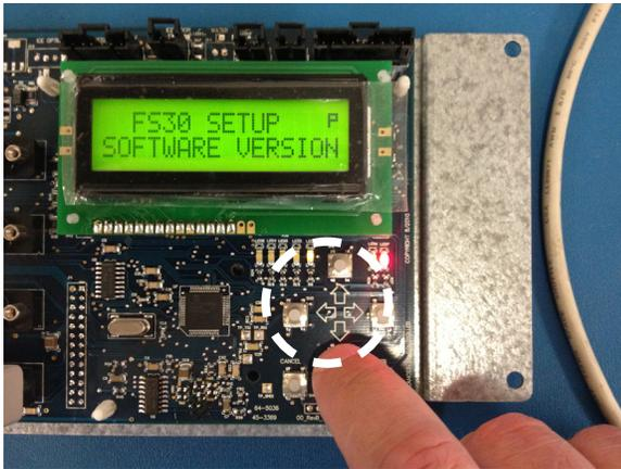
3. Press the enter key to see the current SW versions for the valve boards. By using the up or down arrow button you can change the valve touch pad number to see which software version it has. Verify all valve boards are current by pressing the up or down to view entire list.
