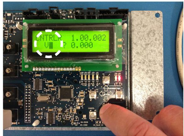
4. If the software version is 3.02 or higher, the valve boards do not need to be replaced.
