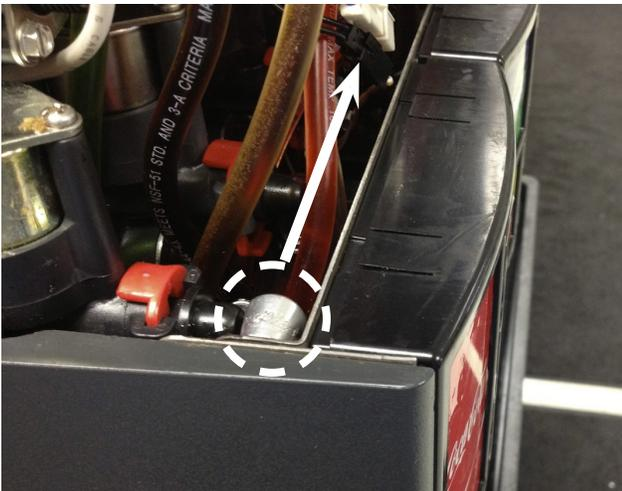
4. Inspect the larger 25-pin cables connected to the Touch Panel. If unit has a short pigtail with four (4) wires, the Valve Cable Harness does **NOT** need to be replaced.
