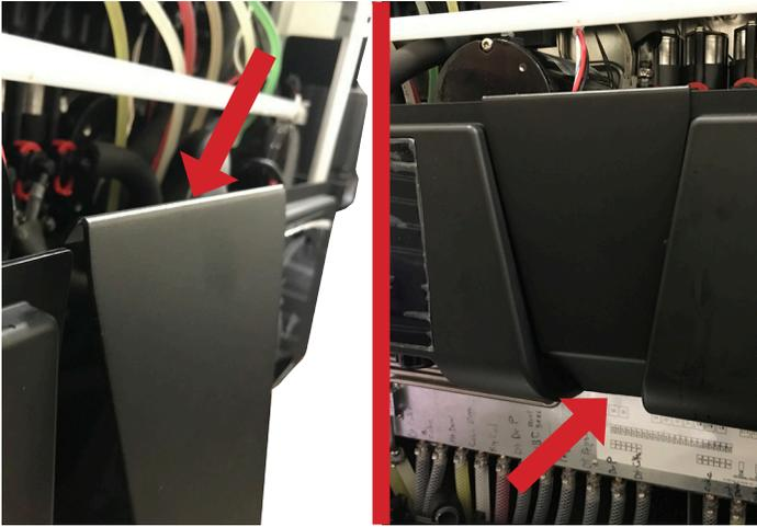
8. Install the right side mounting bracket to ice chute frame of the unit.
