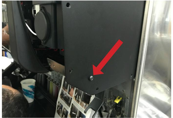
10. Install the right side panel over the right side ice chute, and secure to merchandiser frame using four sheet metal screws supplied in kit.
