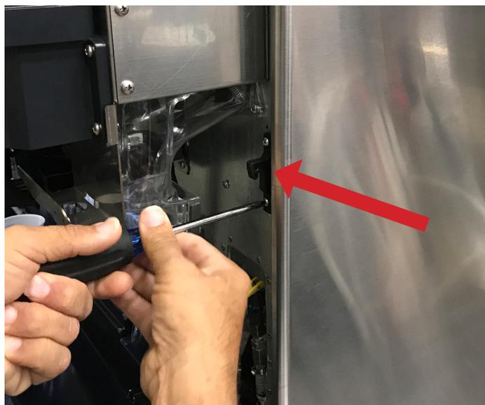
4. Remove the top screws on the outer edge of the dispenser from the left and right side of the unit.
