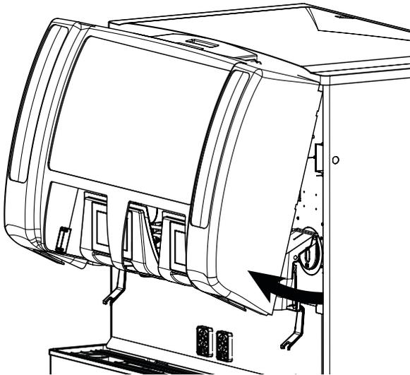
3. Remove the left and right connection tabs, used to connect the original merchandiser to the unit.
