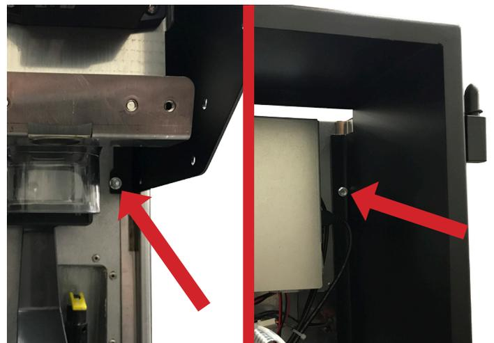
7. Install the center piece, included with kit, in between the two touch pads. Firmly push the center piece back to secure in-between the two touch pads.
