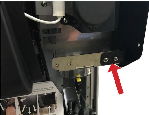
9. Use one of the black sheet metal screws included with kit to secure the merchandiser frame to the mounting bracket.
