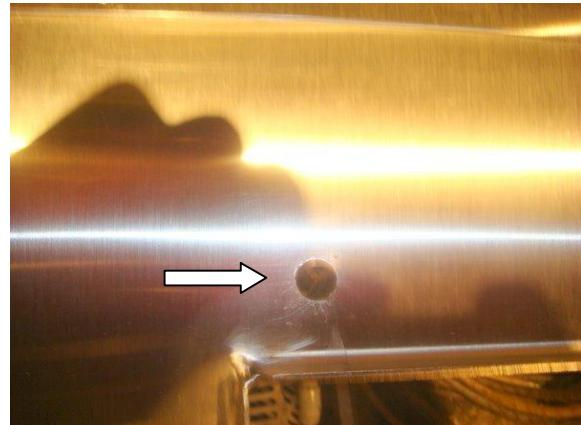
2. Position the dispenser on the counter to align holes with leg threads
