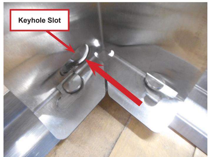
3. With the leg against the inside edge of the top rim, use a rubber hammer or mallet to engage all three (3) rim buttons in the elongated slots.
