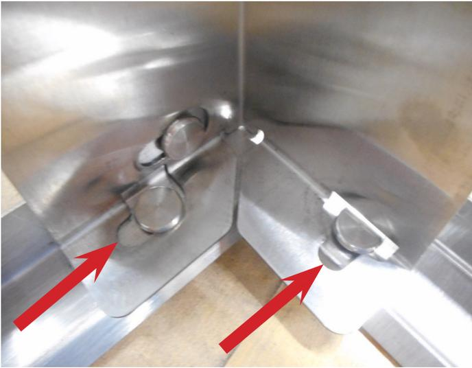
4. Once leg is secured to the inside edge of the top rim, repeat steps 1-3 for the remaining three (3) legs.
