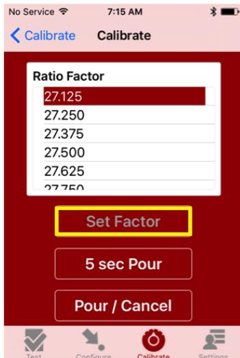
8. Hold the empty ratio cup under the separator and press 5 sec pour. Repeat until the syrup level is even with the water in the ratio cup.
