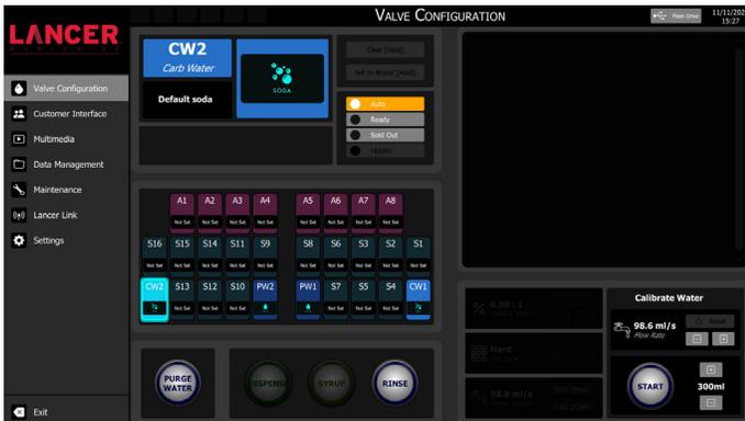
3. Tap the *Purge Water* button to activate purging. Once a steady flow of water is achieved, press the *Stop Purge* button to deactivate.
